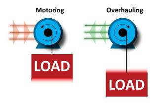
A motor connected to a load will be either "motoring" or "overhauling". A motoring motor is converting electrical energy into mechanical energy as is the case when a load is being lifted. An overhauling motor is being driven by the load and is converting mechanical energy in to electricity, acting as a generator. When the load is being lowered the motor acting as a generator is also acting as a brake for the load.
