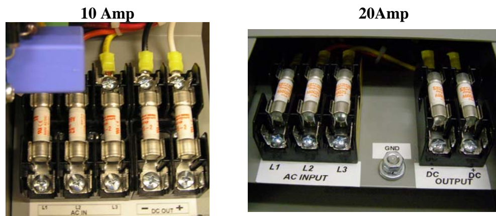
Figure 3-5: M3528 10 Amp and 20 Amp Battery Charger Connections
