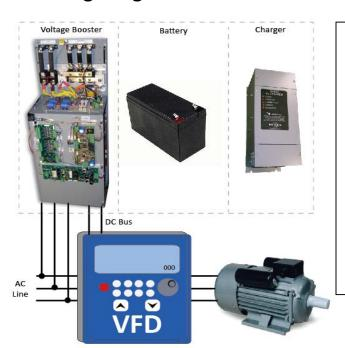
Charger is connected to AC Line Isolation
