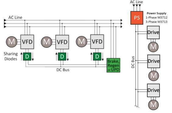
The more general solution is line regeneration, converting the braking energy to AC and sending it to other loads via their normal power inputs. Some larger VFDs are now available with an active
