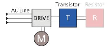
Converting braking energy to heat may be simple, but it has substantial disadvantages. For heavy-duty applications, the resistor may be several times the size of the VFD. All the braking energy is wasted, rather than being used productively to reduce the facility's electricity costs, potentially by
