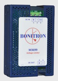
24-Volt Power Supplies are common in nearly every industry. Numerous manufactures offer low cost 24-Volt isolated Power Supplies; however, most only accept a limited input voltage. With the increase in solar and wind applications, many systems need a power supply that can accept voltages as high as 1000VDC. The M3699 serves as a bridge between high voltage DC inputs and 24-Volt Power Supplies.
