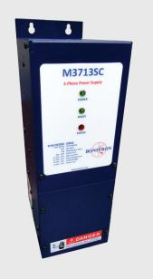
The M3713 can also be used as a building block for 12 and 18 pulse systems using standard VFDs. These systems mitigate harmonics and other power quality issues. Multiple M3713 units used with a phase shifting transformer allows standard drives to meet IEEE 519 compliance.
