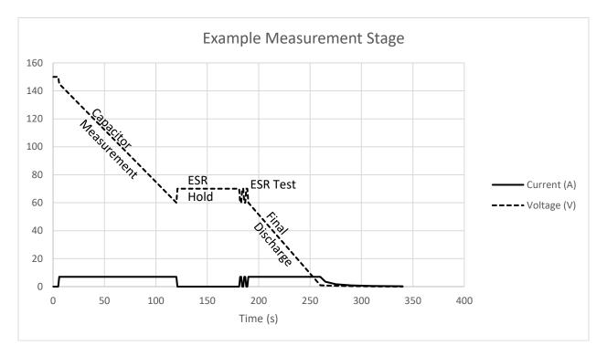
Figure 4-4: M3628UMT Example Measurement Stage
